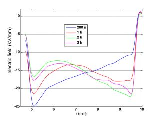
Fig. 6. Measured (PEA) electric field distribution vs. radius for different times, for a MV cable of 4.5mm polarized at -80 kV, and a temperature gradient of  $\Delta T=16^{\circ}C$ .
