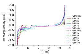
Fig. 4. Net charge density vs. radius for different times of simulation, for the FVM model (lines), and for the FEM model (dotted lines) for a MV cable of 4.5mm thick insulation polarized at -80 kV, and a temperature gradient of  $\Delta$ T=16°C.
