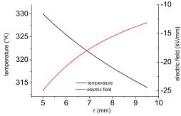
Fig. 1. Temperature distribution and electric field distribution in a MV cable of 4.5mm polarized at -80 kV, with a temperature gradient of  $\Delta T$ =16°C.
