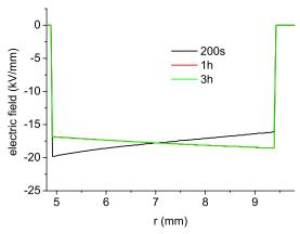
Fig. 5. Electric field distribution vs. radius for different times of simulation, for the macroscopic model and for a MV cable of 4.5mm thick polarized at - 80 kV, and a temperature gradient of  $\Delta T=16^{\circ}C$ .
