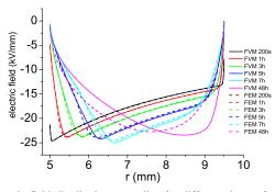
Fig. 3. Electric field distribution vs. radius for different times of simulation, for the FVM model (lines), and for the FEM model (dotted lines) for a MV cable of 4.5mm thick insulation polarized at -80 kV, and a temperature gradient of  $\Delta T$ =16°C.
