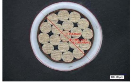
Figure 6. Aeronautic cable observed in the optical microscope
