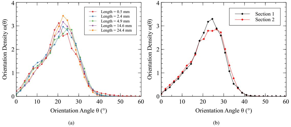
Figure 4: (a) ODF of 5 different lengths (0.5 to 24.4 mm) of a single yarn (410 tpm) : the orientation density functions determined for these different size parameters of the sample show an independency of the location along the yarn axis and a relative accuracy of the measurements down to a length of 0.5 mm. (b) ODF of 2 different locations of a length of 4.5 mm in the same single yarn (410 tpm).
