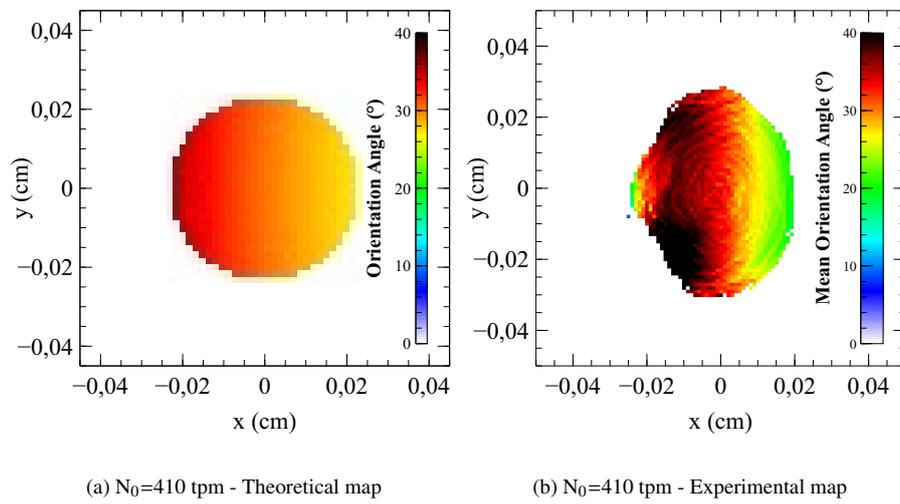
Figure 18: (a) Theoretical (according to equation 12) and (b) experimental spatial distribution of the mean orientation angles in a ply of a 3-ply yarn twisted at 410 tpm. The predicted angle values also show a strong discrepancy.
