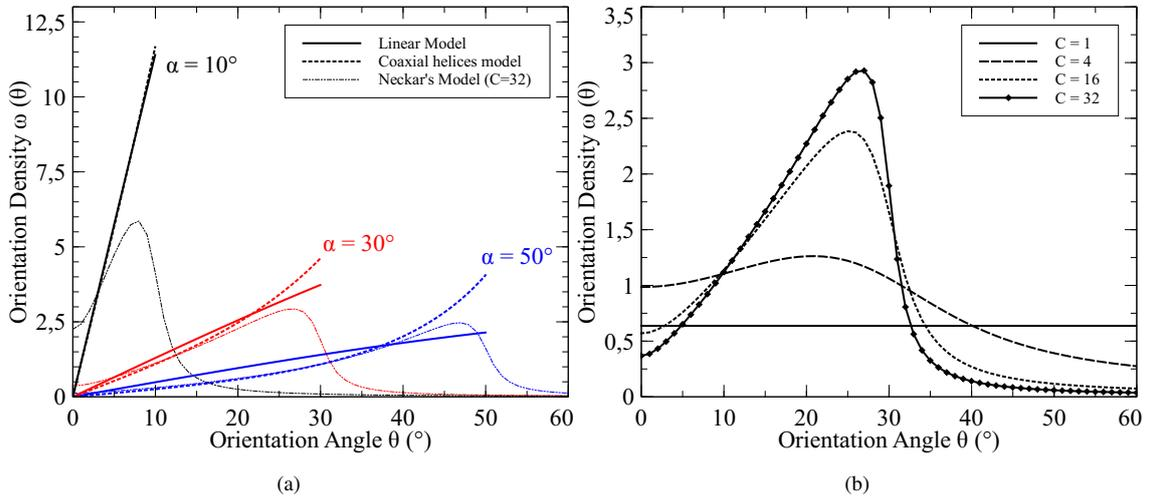
Figure 3: (a) 3 models describe a distribution of fiber orientations in single yarn cross-sections (for 3 values of the yarn surface angle  $\alpha$ ) : the linear model (eq. 7), the perfect coaxial helices model (eq. 9) and Neckar's model (eq. 11). (b) Neckar's model for 4 values of C and a yarn surface angle  $\alpha = 30^\circ$ .
