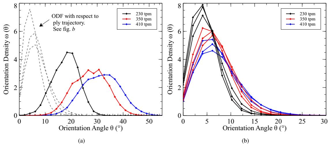
Figure 15: (a) Impact of the twist level on the overall ODF of a 3-ply yarn with respect to the yarn axis. (b) For each level of twist, the ODF of each ply is reported independently with respect its corresponding ply trajectory. Due to the balanced cording process like in the 2-ply yarns, the plies in the same 3-ply yarn show identical ODF.
