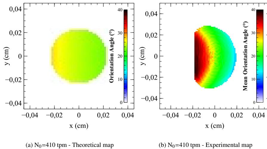
Figure 14: (a) Theoretical (according to eq. 12) and (b) experimental spatial distribution of the mean orientation angles in a ply of a 2-ply yarn twisted at 410 tpm. The predicted angle values show a strong discrepancy.
