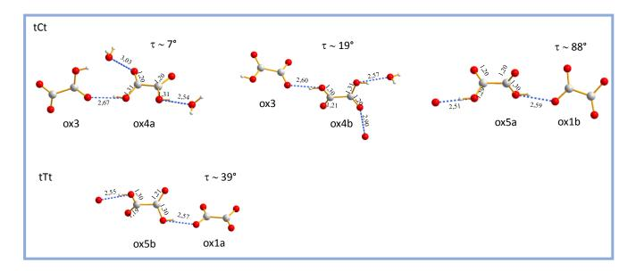
Figure 6: Oxalic acids in the crystal structure of [Th<sub>2</sub>(C<sub>2</sub>O<sub>4</sub>)<sub>3</sub>(TEDGA)<sub>4</sub>][NO<sub>3</sub>][HC<sub>2</sub>O<sub>4</sub>][H<sub>2</sub>C<sub>2</sub>O<sub>4</sub>]<sub>4</sub>.7H<sub>2</sub>O (4).
