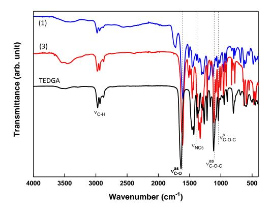
Figure 7: Infrared spectra of TEDGA (in black),  $[Th(TEDGA)_2(C_2O_4)][NO_3]_2[H_2C_2O_4].6H_2O$  (1) (in blue) and  $[Th(TEDGA)_4[NO_3]_4.4H_2O$  (3) (in red).
