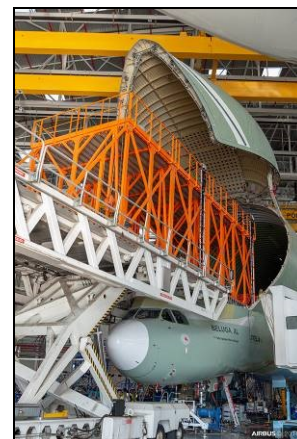
Figure 5: HPJ (orange structure) put in the fuselage
