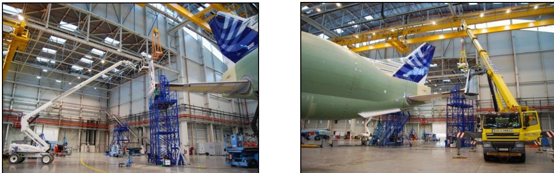
Figure 16 : Auxiliary fins excitation
