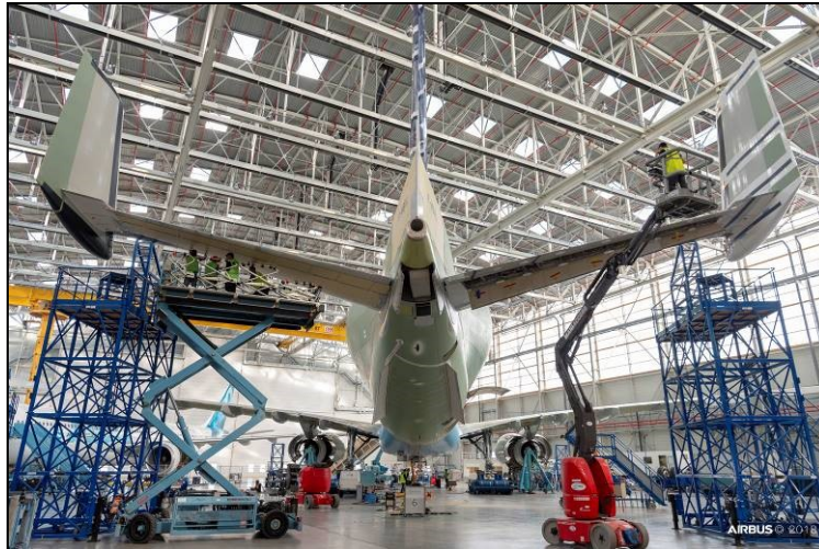
Figure 15 : HTP view with the two auxiliary fins
