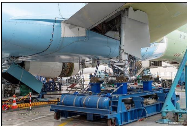
Figure 4 : Main landing gear air spring suspension devices
