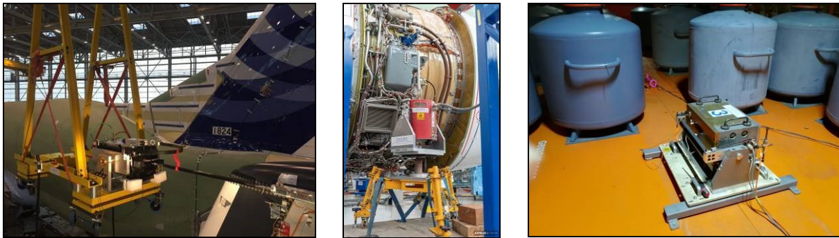
Figure 6 : View of typical exciters used
