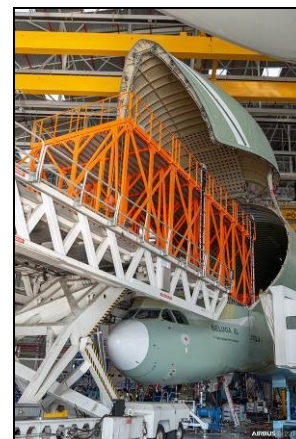
Figure 5: HPJ (orange structure) put in the fuselage
