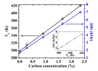
**FIG. 4.** Variations of  $T_C$  and  $\Delta Hr$  of a polycrystalline Mn<sub>5</sub>Ge<sub>3</sub> nano-films versus their C doping concentration. The inset presents the corresponding variation of  $\Delta Hr$  versus  $T_C$  measured in the Mn<sub>5</sub>Ge<sub>3</sub> nano-films containing different C concentrations.
