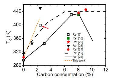
**FIG. 1.** Variations of the Curie temperature ( $T_C$ ) of Mn<sub>5</sub>Ge<sub>3</sub>(C) thin films versus carbon concentration reported in the literature. Our measurements are also plotted for comparison (short dash line). The carbon concentration was measured in each film in our case, while it corresponds to the carbon flux calibration used for deposition in the cases reported in the literature.
