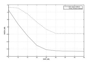
**Fig. 3**. NMSE versus SNR for 4 speech sources and 3 sensors: comparison of the performance of our algorithm with the modified TF-UBSS
