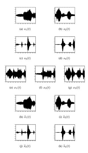
**Fig. 2**. Blind source separation example for 4 speech sources and 3 sensors in instantaneous mixture case: the upper line represents the original source signals, the second line represents the M mixtures and the bottom one represents estimates of sources by our algorithm.
