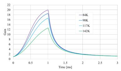
Fig. 10. Small signal gain recorded at 1029.7 nm while pumping the  $Cr^{4+}/Yb^{3+}$ :YAG cosintered ceramic at 5.5kW/cm<sup>2</sup> intensity and single shot, 0.5, 1 and 2 Hz repetition rate. Respective temperatures are 84, 98, 117, 142 K. Helium pressure is 1 bar.
