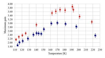
Fig. 8. Maximum gain observed versus  $Cr^{4+}/Yb^{3+}$ :YAG co-sintered ceramic temperature. Extraction wavelength is 1030.3 nm. Pump intensity is 5.5 kW/cm<sup>2</sup> with 1 ms pulse duration. The blue squares are the maximum values observed on Fig. 7 (right), i.e. obtained at 2 Hz with a 150+/-5  $\mu$ m Helium gas gap thickness. The red disks are gain maxima obtained at 5 Hz with a 55+/-5  $\mu$ m gap.
