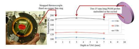
Fig. 5. Left, picture of a Yb:YAG crystal in its mount. The three thermal probes allow temperature measurement at 0, 3 and 7 mm depths. While the amplifier is operated at 1, 2 and 5 Hz, a below 5K axial gradient is observed. Helium pressure is set at 700 mbar, gap thickness at 400  $\mu$ m while pump intensity reaches 5.5 kW/cm<sup>2</sup> homogeneously distributed over the pump area illustrated in red on left picture.
