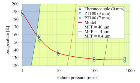
Fig. 6. Yb:YAG ceramic temperature versus helium pressure in a static 400  $\mu$ m thick cell. Isomean free path (MFP) curves are displayed for 40, 4 and 0.4  $\mu$ m. The first one defines the limits between transition (blue) and viscous (green) regimes as defined in section 2.1. Data points were collected while the 5.5 kW/cm<sup>2</sup> pump intensity was delivered at 2 Hz with a 1 ms pulse duration.
