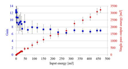
Fig. 11. Left, blue: single pass gain recorded in pulse mode (10 ns / 2 Hz) with the  $Cr^{4+}/Yb^{3+}$ :YAG co-sintered ceramic. Right, Red: Amplified energy in a single pass.
