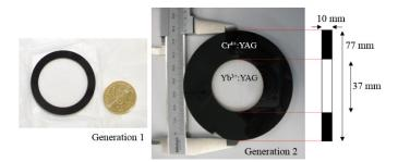
Fig. 3. Illustration of both generations of  $Cr^{4+}/Yb^{3+}$ : YAG co-sintered ceramics.
