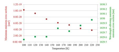
Fig. 9. Maximum emission cross section (red, left scale) and wavelength allowing to reach that maximum (green, right scale) versus temperature. Reaching high cross section values around  $1.10^{-19}$  cm<sup>2</sup> requires a 1029.5 nm source. This graph was derived from data kindly shared by [35].
