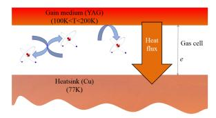
Fig. 1. Schematic illustration of heat transfer processes at work between faces of a helium filled cavity.
