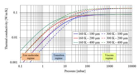
Fig. 2. Thermal conductivity of Helium as a function of pressure for temperature of 160 K (plain lines) and 300 K (dashed lines) and various Helium gap thicknesses.
