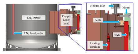
Fig. 4. CAD section view of the low temperature laser head.
