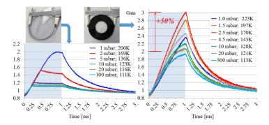
Fig. 7. Single pass gain temporal behavior for two 1 cm thick, 77 mm in diameter Yb:YAG disks operated in the low temperature Lucia amplifier. The 5.5 kW/cm<sup>2</sup> pump is limited at 1 ms duration (blue area) with a 2 Hz repetition rate. The left graph pictures gain curves obtained in the crystal case while the right graph is dedicated to the co-sintered ceramic. The Helium gas gap thickness is 150+/-5 µm.
