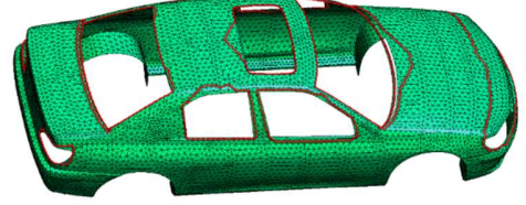
Fig. 4: Mesh of car body and loops found by the circuit solver to take into account multiply connected electric problems
