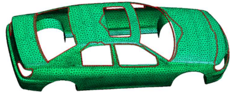
Fig. 4: Mesh of car body and loops found by the circuit solver to take into account multiply connected electric problems
