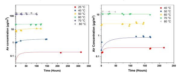
Figure 3. The emission of DiNP (left) from  $VF_1$  and DnOP (right) from  $VF_2$  at different temperatures in the micro-chamber.
