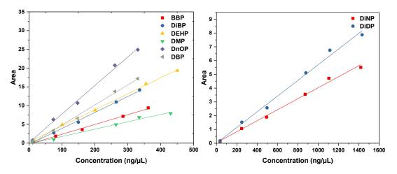
Figure 2. Linearity profile of the calibration curves of eight selected phthalates using the developed ATD-GC-MS method.
