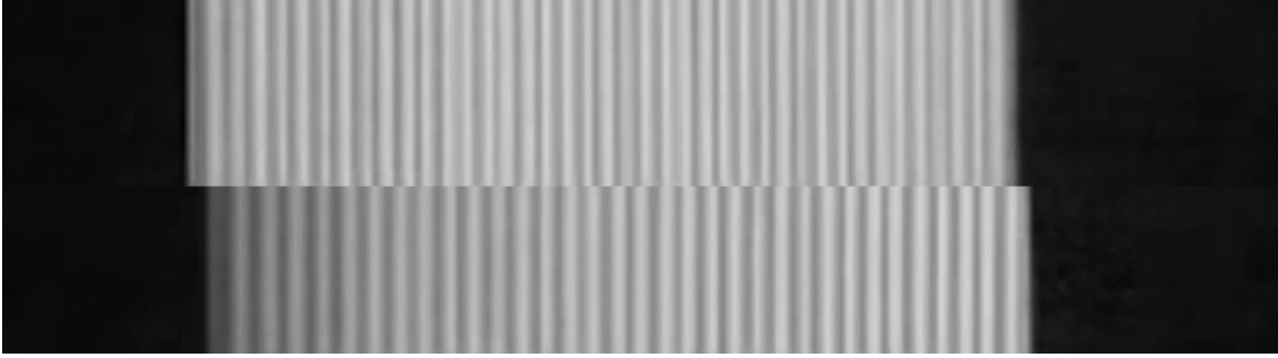
Figure 2: SFT fringe pattern detail of two arbitrary frames of a recording of the rigid hydrofoil. The fringe deformation of the pattern is visible as well as the changes in the apparent surface length, the latter is a result of the two dimensional camera view and the three dimensional oscillation and deformation. The black areas are regions without a surface and so without projection, which irritate the processing algorithm.
