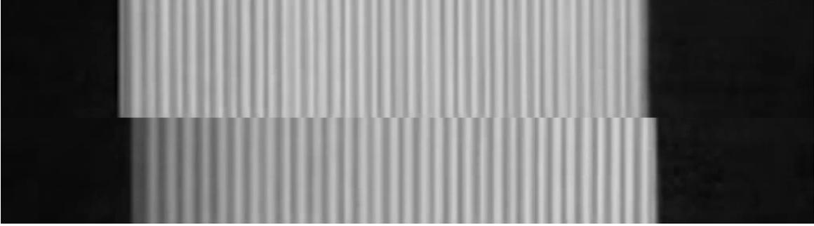
Figure 2: SFT fringe pattern detail of two arbitrary frames of a recording of the rigid hydrofoil. The fringe deformation of the pattern is visible as well as the changes in the apparent surface length, the latter is a result of the two dimensional camera view and the three dimensional oscillation and deformation. The black areas are regions without a surface and so without projection, which irritate the processing algorithm.
