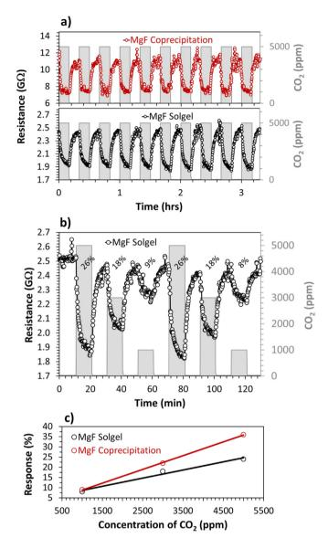
**Fig. 6.** (a) Change in resistance at 300  $^{\circ}$ C of co-precipitated and sol gel combusted magnesium ferrite samples in the presence of 5000 ppm CO<sub>2</sub>. (b) Variation of the resistance at 300  $^{\circ}$ C with concentration for Mg ferrite sol-gel combusted sample. (c) Variation of the resistance at 300  $^{\circ}$ C as a function of the CO2 concentration for both samples.
