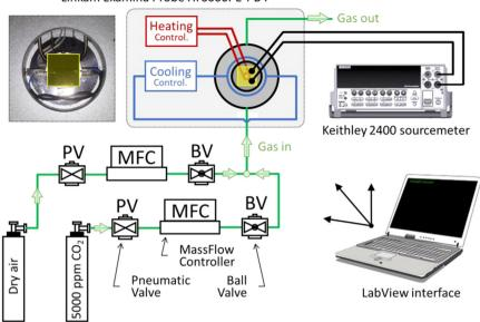
Fig. 1. Schematic of the CO<sub>2</sub> sensing set up.
