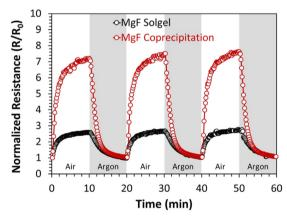
Fig. 5. Variation of the response  $R/R_0$  at 300 °C of magnesium ferrite samples co-precipitated and sol-gel combusted in the presence of air and argon.
