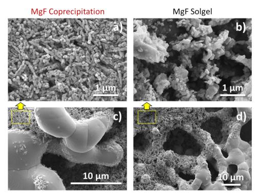
Fig. 3. SEM micrograph of magnesium ferrite powders prepared by co-precipitation [a), c)] and sol gel combustion [b), d)] coated on porous silver electrode for electrical and gas sensing measurements.
