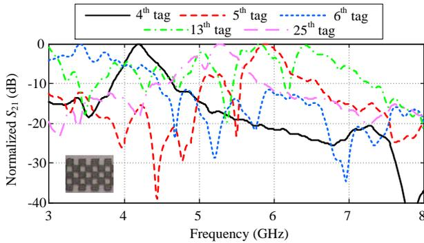
Fig. 7. First measurement of  $S_{21}$  in the form of windowed FD responses for selected chipless tags from the population of thirty chipless tags. Inset: corresponding zoom photograph of the inkjet-printed five squares check pattern.
