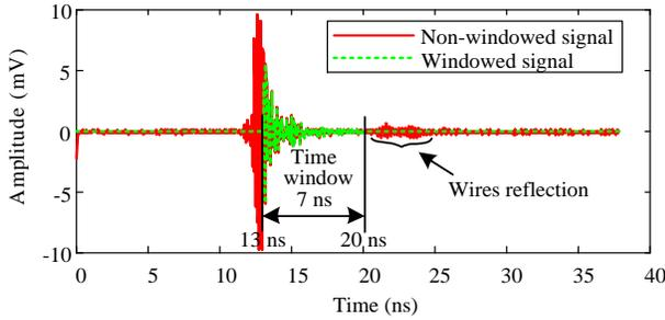
Fig. 6. Time windowing to discard the structural mode and to extract the antenna mode of  $S_{21}$  of first squares check patterned tag measured with IR-UWB reader. The start time of time window is 13 ns and the duration of time window is 7 ns.
