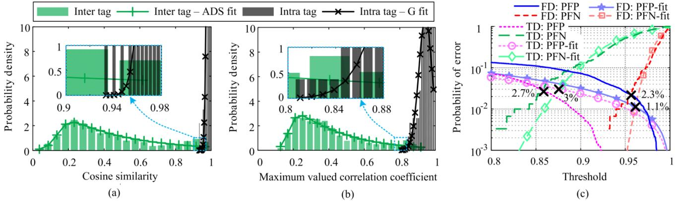
Fig. 9. Similarity analysis for the inkjet-printed PET five squares patterned tags with  $d_s = 70.7 \mu\text{m}$  measured using IR-UWB chipless reader. (a) Intra- and inter-tag cosine similarity PDF distributions for FD analysis. (b) Intra- and inter-tag maximum valued correlation coefficient PDF distributions for TD analysis. (c) Probabilities of false positive and false negative for both FD and TD analyses.
