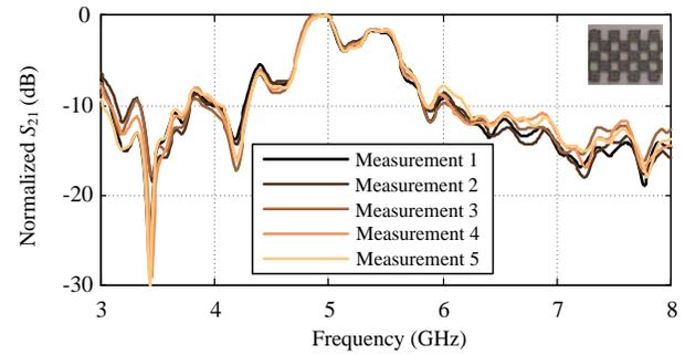
Fig. 8. Five repetitive measurements of  $S_{21}$  in the form of windowed FD responses for first tag from five squares check patterned C-folded scatterer tags population using IR-UWB chipless reader. Inset: corresponding zoom photograph of the inkjet-printed pattern.
