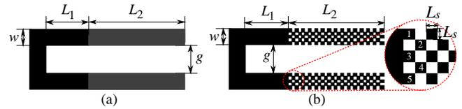
Fig. 2. Layouts of the C-folded scatterers. (a) Conventional design of the C-folded scatterer. (b) Optimized design of the C-folded scatterer exhibiting five squares check pattern.  $L_1 = 5.35$  mm,  $L_2 = 17.15$  mm,  $w = 2$  mm,  $g = 3.5$  mm, and length (and width) of each square geometry  $L_s = 0.4$  mm.
