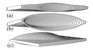
FIG. 2. Perspective view of the iso-surface  $\varphi = 0.5$  (that can be considered as the crack surface) at different times of a branching event for a thin system  $(T \approx 12w_{\varphi})$  with tractionfree boundary conditions at  $z = \pm T/2$ . (a) A tip splitting instability is initiated at the middle of the crack front and (b) spreads along the crack front. (c) represents the same state as (b) seen from the rear crack front.
