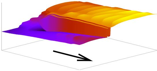
FIG. 5. A fracture surface with an echelon crack. The whole thickness of the material is shown and the secondary branches have been removed for clarity. Traction-free boundary conditions at  $z = \pm T/2$  were used in the simulation. The arrow indicates the main direction of crack propagation.
