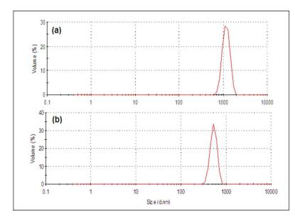
Fig. 3. Zetasizer of CuO (a) and CuO@Ag $^{0}$  (b).
