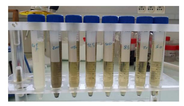
Figure. 10: Change in solution turbid for various concentration of CuO@Ag<sup>0</sup>.
