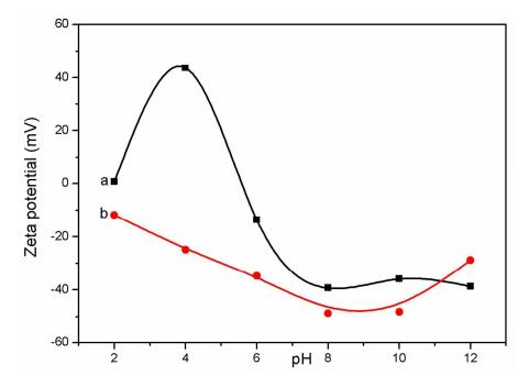
Fig. 5. Zeta potential of CuO (a) and CuO@Ag<sup>0</sup> (b) for different pH values.
