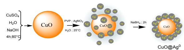
Scheme 1. Synthetic route for CuO@Ag<sup>0</sup> core-shell.
