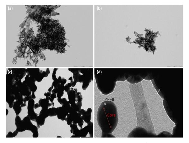
Fig. 2. TEM image of synthesized CuO (a, b) and CuO@Ag<sup>0</sup> (c, d).
