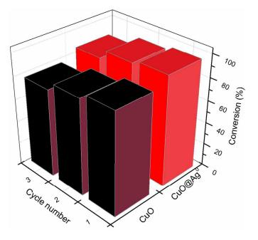
**Fig.9**. Conversion yield of 4-NP after repetitive catalytic tests of CuO and CuO@Ag<sup>0</sup> at room temperature. Reaction conditions. 4-NP = 2.5mM, NaBH<sub>4</sub> = 0.2 M, [CuO]=0.10 mg/L,
