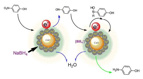
Scheme 2. Proposed mechanism for 4-NP reduction with  $CuO@Ag^0$  as catalyst.
