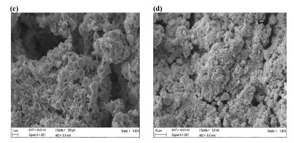
Fig. 1. SEM image of synthesized CuO (a, b) and CuO@Ag<sup>0</sup> (c, d).
