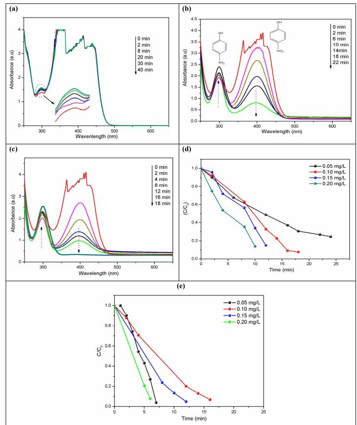
Fig. 8. UV–Vis absorption spectra for the reduction of 4-NP at room temperature with NaBH<sub>4</sub>
