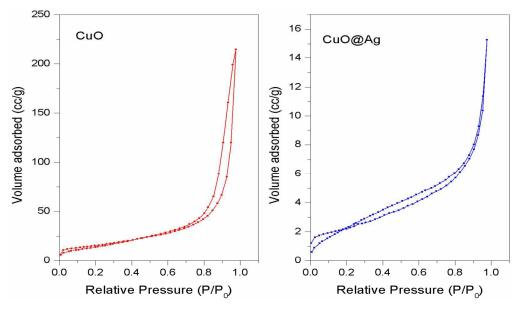
Fig. 4. Nitrogen adsorption-desorption isotherms of CuO and CuO@Ag<sup>0</sup>.
