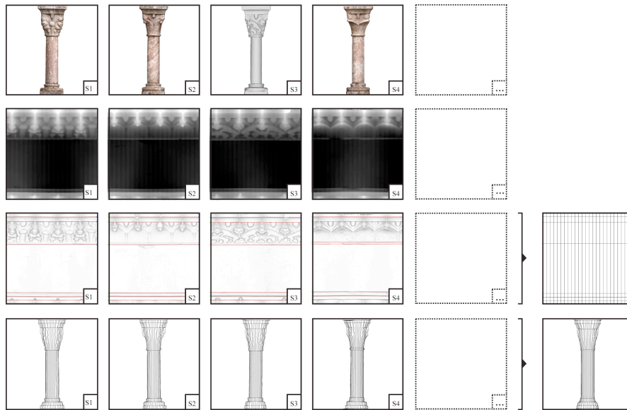
Fig. 6. First 4 columns of the collection: Polygonal mesh, depth map, discontinuities, simplified geometric reconstruction and average values (right side).
