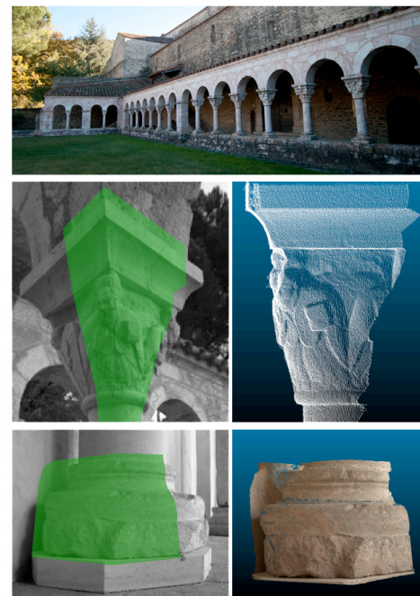
Fig. 1. Masks and point clouds from the photogrammetric acquisition of the columns of Saint-Michel de Cuxa
