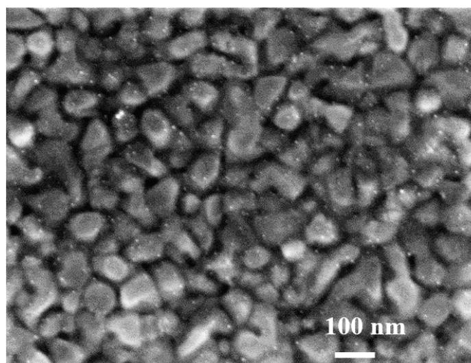
**Figure 2.** Field emission gun scanning electron microscopy (FEG-SEM) image of the gold electrode functionalized by silver nanoparticles ( $E_{\text{Au/AgNPs}}$ ). The functionalization conditions correspond to a silver precursor concentration of  $0.04 \text{ mol}\cdot\text{L}^{-1}$ , and a hydrogenolysis duration of 1 min. The image shows small white dots which represent the very small AgNPs and the Au grains (average size ca. 150 nm) of the gold electrode ( $E_{\text{Au}}$ ).
