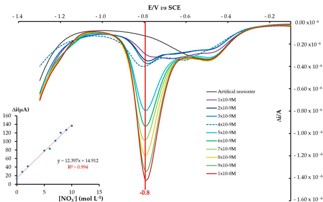
**Figure 4.** Square wave voltammograms obtained in aerated artificial seawater for successive nitrate ions concentrations on the gold electrode functionalized by *in situ* metalorganic deposition of silver nanoparticles ( $E_{Au/AgNPs}$ ). Inset: Calibration plot based on the peak current ( $\Delta i$ ).  $i$  vs.  $[NO_3^-]$  and linear regression.
