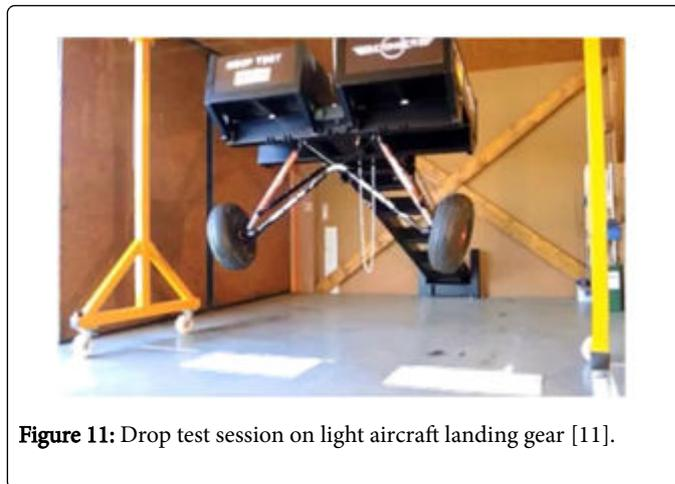
Figure 11: Drop test session on light aircraft landing gear [11].
