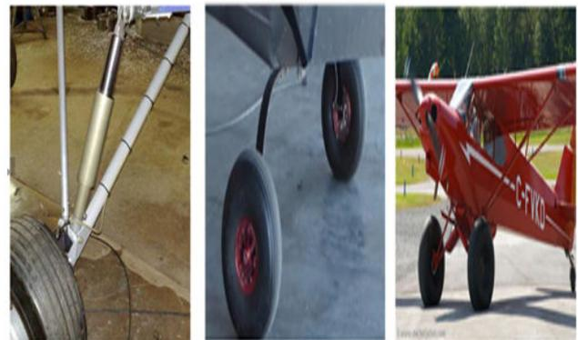
**Figure 1:** Landing gears studied: (a) Landing gear with damper [1], (b) Landing gear with steel struts, (c) Landing gear with Sandow cords [3].
