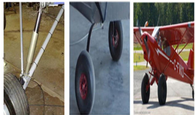
Figure 1: Landing gears studied: (a) Landing gear with damper [1], (b) Landing gear with steel struts, (c) Landing gear with Sandow cords [3].
