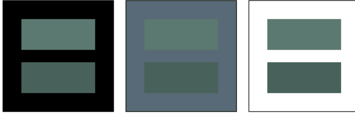
Figure 5: The crispning effect (see text) used to refute Resnikoff's Axiom 6 about the invariance of the perceptual color metric with respect to changes of background illuminations.
