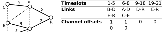
Fig. 1. Example topology and the corresponding LOST scheduling.
