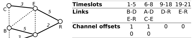
Fig. 1. Example topology and the corresponding LOST scheduling.
