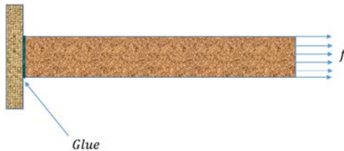
Fig. 2. A simple rod with damaged interface on its left end.
