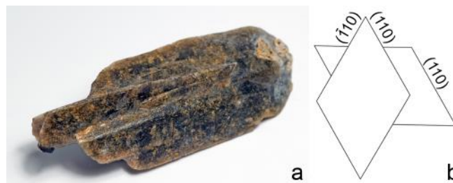
846 Figure 7: Prism (110) twin (#13543, 49.4 x 18.3 x 10.8 mm), (a) photo, (b) theoretical sketch 847 showing the orientation of both individuals (view along [001] ).
