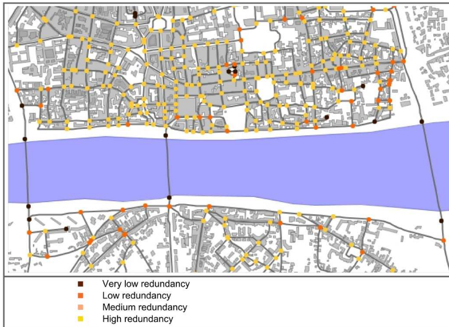
362 363 Fig. 7. Orleans (France) road network redundancy analysis shows the weak redundancy of this 364 network close to bridges (source: Lhomme et al., 2013) 365
