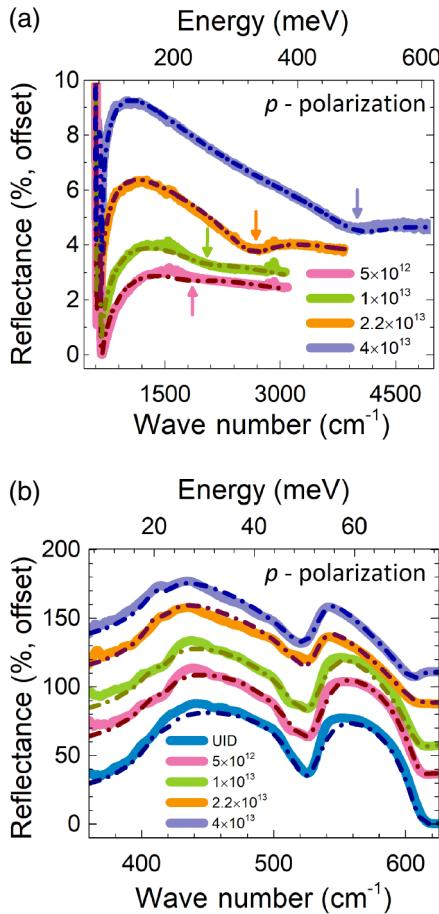
FIG. 3. IR reflectance results. (a) All doped samples in the study under *p* polarization, offset for clarity. Arrows indicate the presence of the MSP. (b) Enlarged view of the reststrahlen band also under *p* polarization, offset for clarity. The best fit for each spectra is overlaid on the experimental data in all the figures (dashed lines). Legends show the values of  $n_{2D}$  extracted from reflectance experiments in units of  $\text{cm}^{-2}$  (see Ref. [24]).
