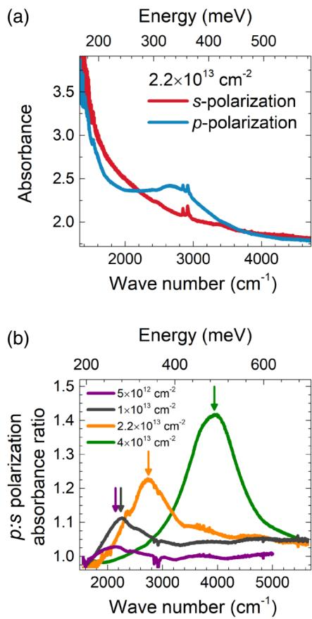
FIG. 4. MSP absorption. (a) Absorbance spectra of sample C under *p* and *s* polarization of the incident light in a 45° multipass waveguide configuration. (b) *p:s* polarization absorbance ratio for all the doped samples in the study. Legends show the experimental values of  $n_{2D}$ .
