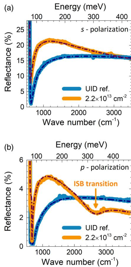
FIG. 2. IR reflectance measurements and fits. (a) Sample *C* and its equivalent undoped reference under *s* polarization of the incident light. (b) Same as (a) but under *p* polarization. The best fit for each spectra is overlaid on the experimental data in all the figures (dashed lines). Legends show the values of  $n_{2D}$  extracted from reflectance experiments in units of  $\text{cm}^{-2}$  (see Sec. II and Ref. [24]).
