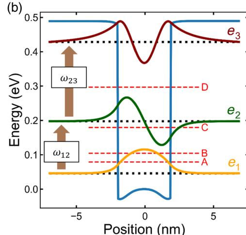
FIG. 1. Details on the samples in this work. (a) Schematic of the multiple quantum well structures presented. The table shows the different doping levels and schemes employed. (b) Potential profile of one of the QWs in sample *D* calculated from the self-consistent solution of the Schrödinger and Poisson equations. Wave functions are offset to match their respective energy levels. Red lines indicate the Fermi energy for all samples. The allowed ISB transitions are also indicated.
