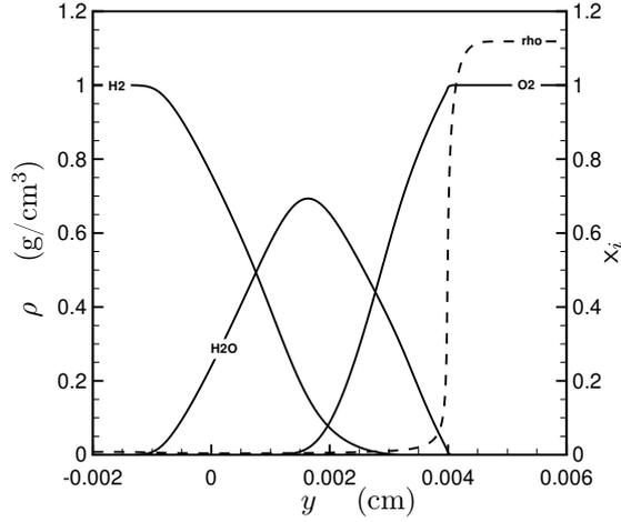
Figure 9: Mass density  $\rho$  and mole fractions of major species in a counterflow  $\text{H}_2\text{-O}_2$  diffusion flame, with  $T_+ = 100$  K,  $y_{\text{O}_2+} = 1$ ,  $T_- = 300$  K,  $y_{\text{H}_2-} = 1$ ,  $\alpha = 10000$  s $^{-1}$ , and  $\bar{p} = 100$  atm.
