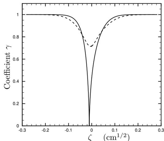
Figure 1: Coefficient  $\gamma$  in a mixing layer at  $\bar{p} = 100$  atm;  $- - T_{\pm} = 160$ ;  $— T_{\pm} = 122$  K
