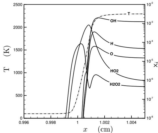
Figure 5: Temperature  $T$  and mole fractions of minor species in a freely propagating  $\text{H}_2$ -Air stoichiometric flame structure at  $\bar{p} = 100$  atm and  $T^{\text{fr}} = 100$  K.
