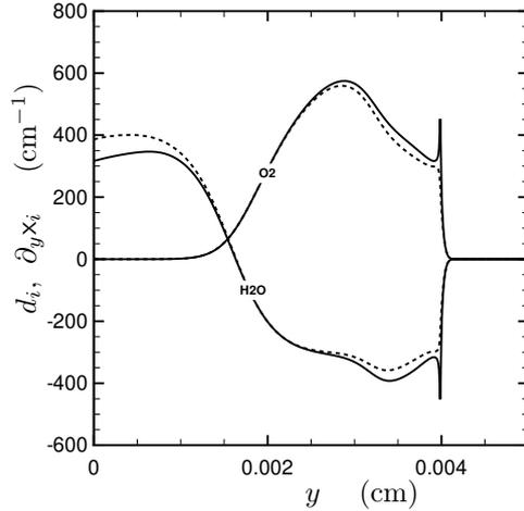
Figure 11: Oxygen and water diffusion driving forces in a counterflow H<sub>2</sub>-O<sub>2</sub> diffusion flame, with  $T_+ = 100$  K,  $y_{O_2+} = 1$ ,  $T_- = 300$  K,  $y_{H_2-} = 1$ ,  $\alpha = 10000$  s<sup>-1</sup>,  $\bar{p} = 100$  atm; —  $d_i$ ; —  $\partial_y x_i$ .
