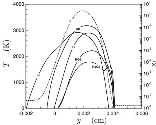
Figure 10: Temperature  $T$  and mole fraction of minor species in a counterflow  $\text{H}_2\text{-O}_2$  diffusion flame, with  $T_+ = 100$  K,  $y_{\text{O}_2+} = 1$ ,  $T_- = 300$  K,  $y_{\text{H}_2-} = 1$ ,  $\alpha = 10000$  s $^{-1}$ , and  $\bar{p} = 100$  atm.
