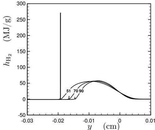
Figure 13: Hydrogen partial enthalpies in supercritical H<sub>2</sub>-O<sub>2</sub> diffusion flames, with  $T_- = 100$  K,  $y_{\text{O}_2^-} = 1$ ,  $T_+ = 300$  K,  $y_{\text{H}_2^+} = 1$ ,  $\alpha = 1000$  s<sup>-1</sup> and pressures  $p^\infty = 51, 70, 90$  atm.
