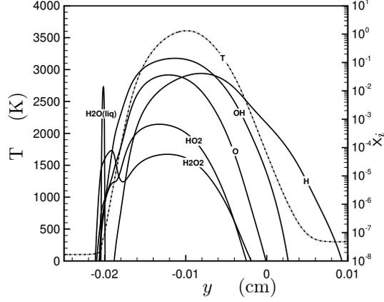
Figure 15: Temperature  $T$  and species mole fractions in a diffuse interface  $\text{H}_2\text{-O}_2$  diffusion flame at  $p^\infty = 45$  bars with  $T_- = 100$  K,  $y_{\text{O}_2^-} = 1$ ,  $T_+ = 300$  K,  $y_{\text{H}_2^+} = 1$ ,  $\alpha = 1000$  s $^{-1}$
