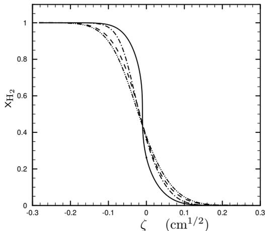
Figure 2: Hydrogen mole fraction in a mixing layer at  $\bar{p} = 100$  atm; —  $T_{\pm} = 122$  with nonideal diffusion; - -  $T_{\pm} = 122$  with ideal diffusion; - .  $T_{\pm} = 160$  with nonideal diffusion; . .  $T_{\pm} = 160$  with ideal diffusion
