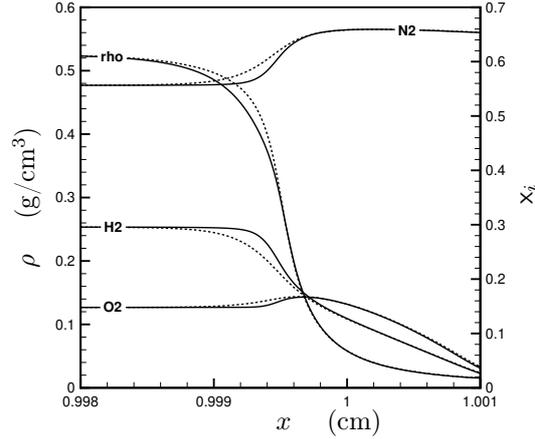
Figure 6: Impact of transport nonidealities in a freely propagating H<sub>2</sub>-Air stoichiometric flame at  $\bar{p} = 100$  atm and  $T^{\text{fr}} = 100$  K; — nonideal diffusion; - - ideal diffusion.
