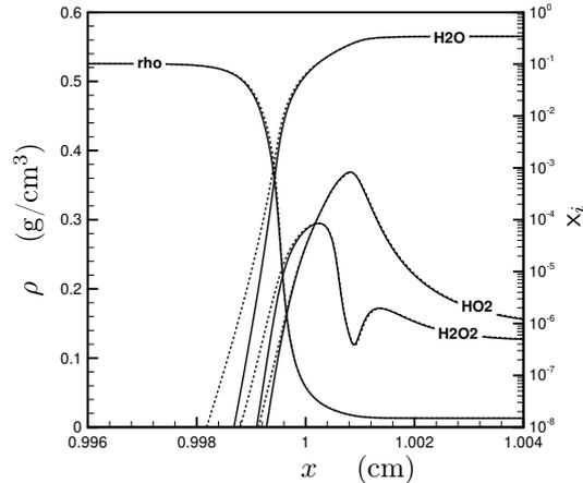
Figure 8: Impact of high pressure correctors of binary diffusion coefficients in a freely propagating H<sub>2</sub>-Air stoichiometric flame at  $\bar{p} = 100$  atm and  $T^{\text{fr}} = 100$  K; — nonideal diffusion; - - ideal diffusion.
