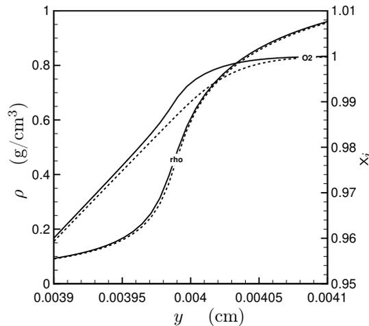
Figure 12: Density  $\rho$  and oxygen mole fraction in a counterflow H<sub>2</sub>-O<sub>2</sub> diffusion flame, with  $T_+ = 100$  K,  $y_{O_2+} = 1$ ,  $T_- = 300$  K,  $y_{H_2-} = 1$ ,  $\alpha = 10000$  s<sup>-1</sup>,  $\bar{p} = 100$  atm; — nonideal diffusion; - - ideal diffusion.
