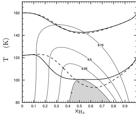
Figure 3: Phase diagram with mixing layer trajectories at  $\bar{p} = 100$  atm,  $T_{\pm} = 160$  K and  $T_{\pm} = 122$  K; — nonideal diffusion; - - ideal diffusion.
