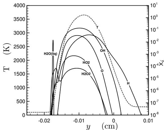
Figure 14: Temperature  $T$  and species mole fractions in a diffuse interface H<sub>2</sub>-O<sub>2</sub> diffusion flame at  $p^\infty = 60$  bars with  $T_- = 100$  K,  $y_{\text{O}_2^-} = 1$ ,  $T_+ = 300$  K,  $y_{\text{H}_2^+} = 1$ ,  $\alpha = 1000$  s<sup>-1</sup>
