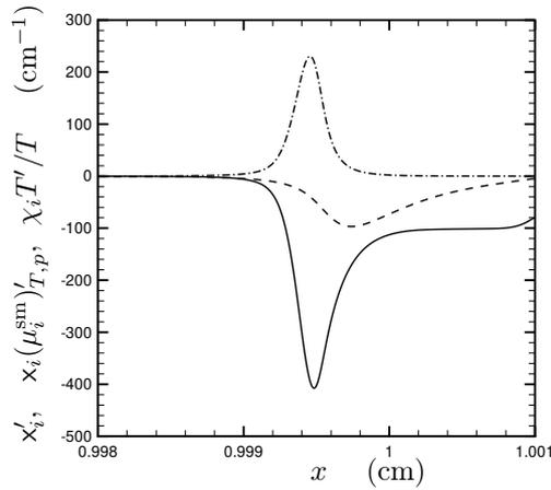
Figure 7: Hydrogen diffusion driving forces in a freely propagating H<sub>2</sub>-Air stoichiometric flame at  $\bar{p} = 100$  atm and  $T^{\text{fr}} = 100$  K; —  $\chi'_i$ ; - -  $\chi_i(\mu_i^{\text{sm}})'_{T,p}$ ; - ·  $\chi_i T'/T$ .
