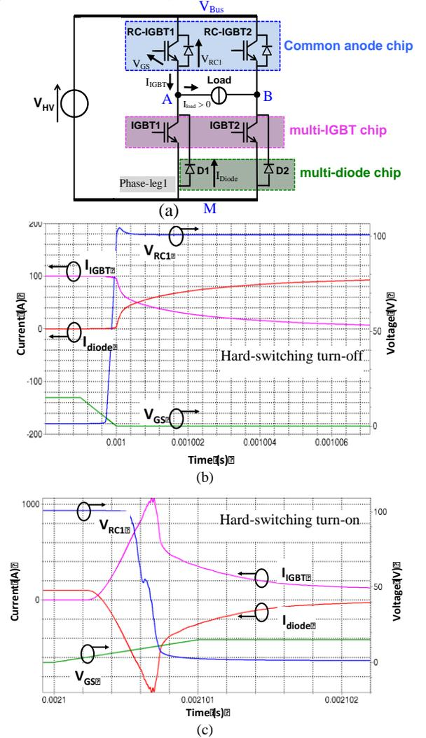
Fig. 15. Mixed-mode Sentaurus<sup>TM</sup> 2D simulations of the single-phase inverter: (a) H-bridge circuit consisting of the three multi-terminal chips, (b) zoom into the turn-off of RC-IGBT1, (c) zoom into the turn-on of RC-IGBT1.
