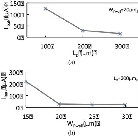
Fig. 14. Qualitative leakage current evaluation in the OFF-state diode section as function of: (a) distance  $L_D$ , (b)  $P^+$  wall width  $W_{Pwall}$ .  $P_{wall}$  doping =  $5 \times 10^{19}\ \text{cm}^{-3}$ .
