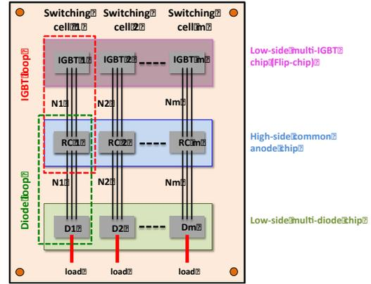
Fig. 3. Proposed assembly for the integrated power converter.
