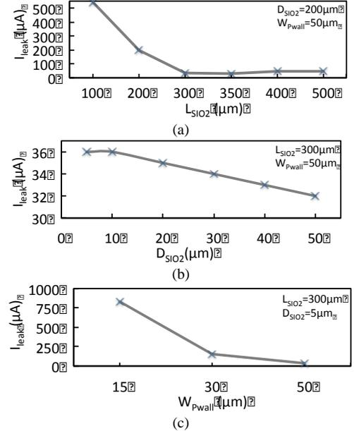
Fig. 11. Qualitative evaluation of the leakage current in the OFF-state IGBT section as function of: (a) the length of the backside oxide trench ( $L_{SiO_2}$ ), (b) the depth of the backside oxide trench ( $D_{SiO_2}$ ) and (c) the width of the  $P^+$  wall ( $W_{Pwall}$ ),  $P_{wall}$  doping =  $5 \times 10^{19} \text{cm}^{-3}$ .
