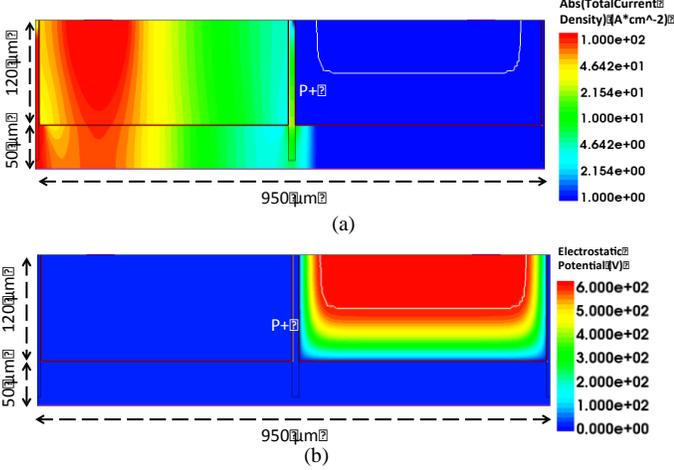
Fig. 13. 2D simulation results of the common anode multi-diode chip: (a) current density distribution and (b) equipotential lines distribution.  $W_{Pwall} = 20\ \mu\text{m}$ ,  $P_{wall}$  doping =  $5 \times 10^{19}\ \text{cm}^{-3}$ .
