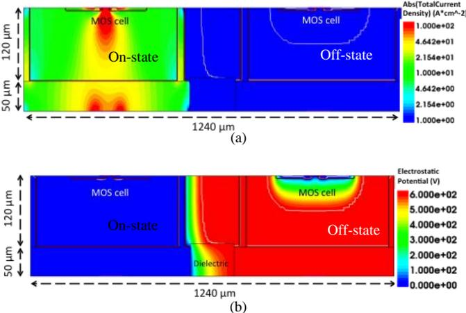
Fig. 10. 2D simulation results of the common cathode multi-IGBT chip: (a) current density distribution and (b) equipotential lines distribution. Case where  $L_{SiO_2} = 300 \mu\text{m}$ ,  $D_{SiO_2} = 5 \mu\text{m}$  and  $W_{Pwall} = 20 \mu\text{m}$ ,  $P_{wall}$  doping =  $5 \times 10^{19} \text{cm}^{-3}$ .
