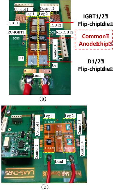
Fig. 19. (a) Realized 3-chip inverter using one common anode chip (11.2mm X 4.9mm X300 $\mu$ m), two IGBTs and two diodes (SIDC30D120H8). (b) Realized reference inverter using four RC-IGBT chips (5.6mm X 4.9mm X300 $\mu$ m). (Capacitor: Kemet C1812V104KCRACU /0.1 $\mu$ F/500V/X7R)
