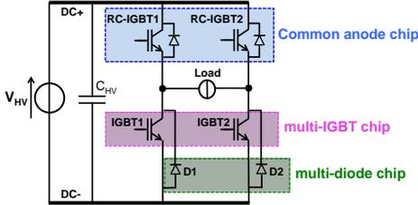
Fig. 2. Principle of the three-chip integration concept.
