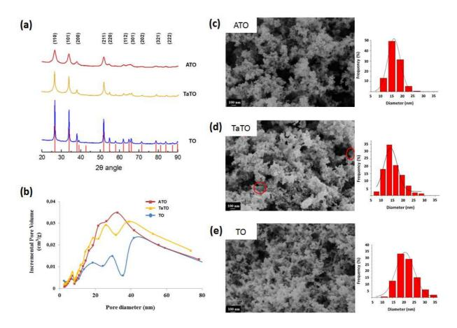
**Figure 2:** X-ray diffraction patterns (a), pore size distribution (b), SEM images (Magnification of the images = 50000 X) and associated primary particle size distributions (c) for pure and doped SnO<sub>2</sub> aerogels (Red bars in (a) correspond to the pattern of the rutile structure of tin oxide <sup>45</sup> JCPDS 14-1445).
