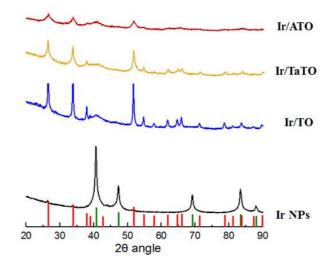
Figure 4. X-ray diffractograms of Ir NPs (black), Ir/TO (blue), Ir/ATO (dark red) and Ir/TaTO (yellow). Red bars correspond to the rutile structure of pure TO and green color ones correspond to Ir(0) pattern.<sup>46, 53</sup>
