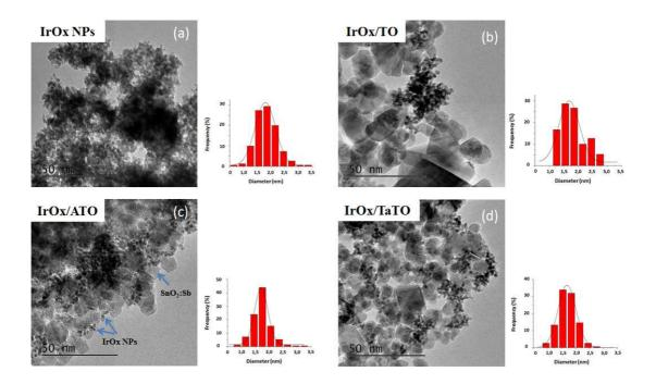
Figure 5. TEM images of (a)  $IrO_x$  NPs, (b)  $IrO_x$ / TO, (c)  $IrO_x$ / ATO and (d)  $IrO_x$ /TaTO and associated  $IrO_x$  particle size
