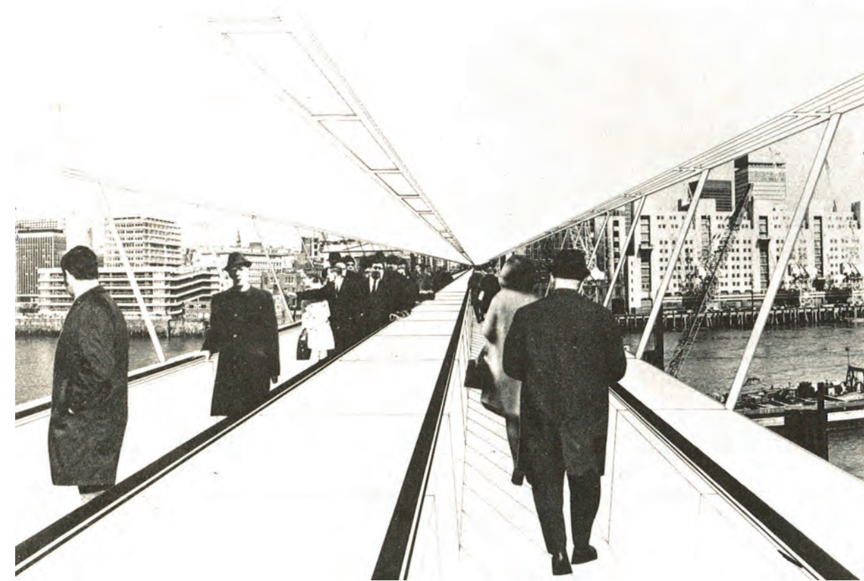
The immobile walker. Speedway links crossing the Thames. "Interior view along system, which can carry up to 10,000 people an hour in each direction..." (B. Richards, 1976)
