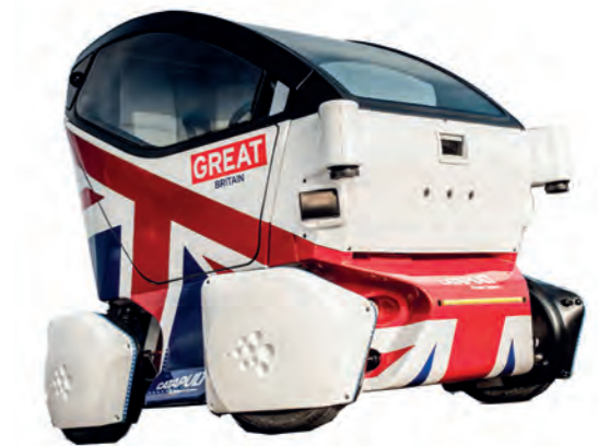
Catapult, “driverless pod” two-seat automated transporter being demonstrated in Greenwich, 2015
