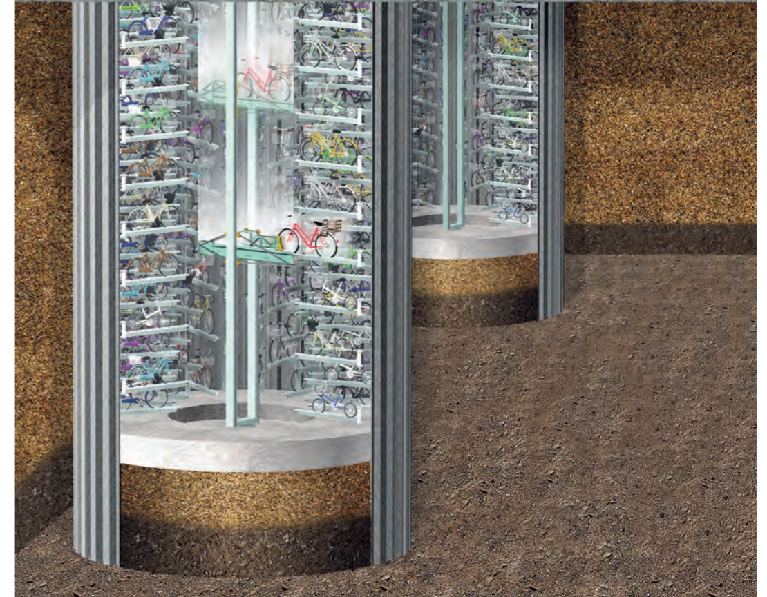
Giken underground eco-cycle parking system, Tokyo
