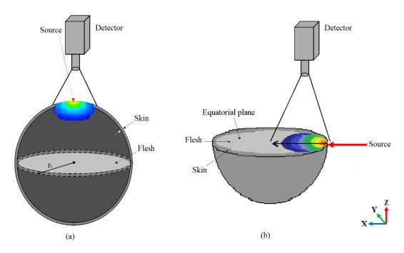
**Figure 1.** Apple models and imaging-tissue setups used for the Monte Carlo simulations. (a) Whole apple assimilated to a sphere (flesh) surrounded by a thin layer of tissue (skin), and observed over its top curved boundary; (b) Half-cut spherical apple model observed over its equatorial plane. In both cases, the Gaussian beam size of the incident light source is  $2\omega_0 = 1$  mm.
