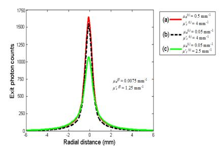
**Figure 6.** Diffuse reflectance profiles plotted as a function of the radial distance  $\rho = \sqrt{X^2 + Y^2}$ , and corresponding to the three generated images (**a**, **c**) displayed in Figure 5.
