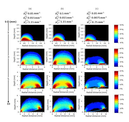
**Figure 8.** Source-detector sensitivity profiles computed for a skin thickness  $d = 80 \mu m$ , four source-detector distances S-D = 1 mm, 3 mm, 5 mm and 10 mm (horizontal columns), and different combinations of optical properties  $\mu'_s(s) = 4 \text{ mm}^{-1} - \mu_a(s)$ ;  $\mu_a(f) - \mu'_s(f)$  (vertical columns (**a-b-c**)).
