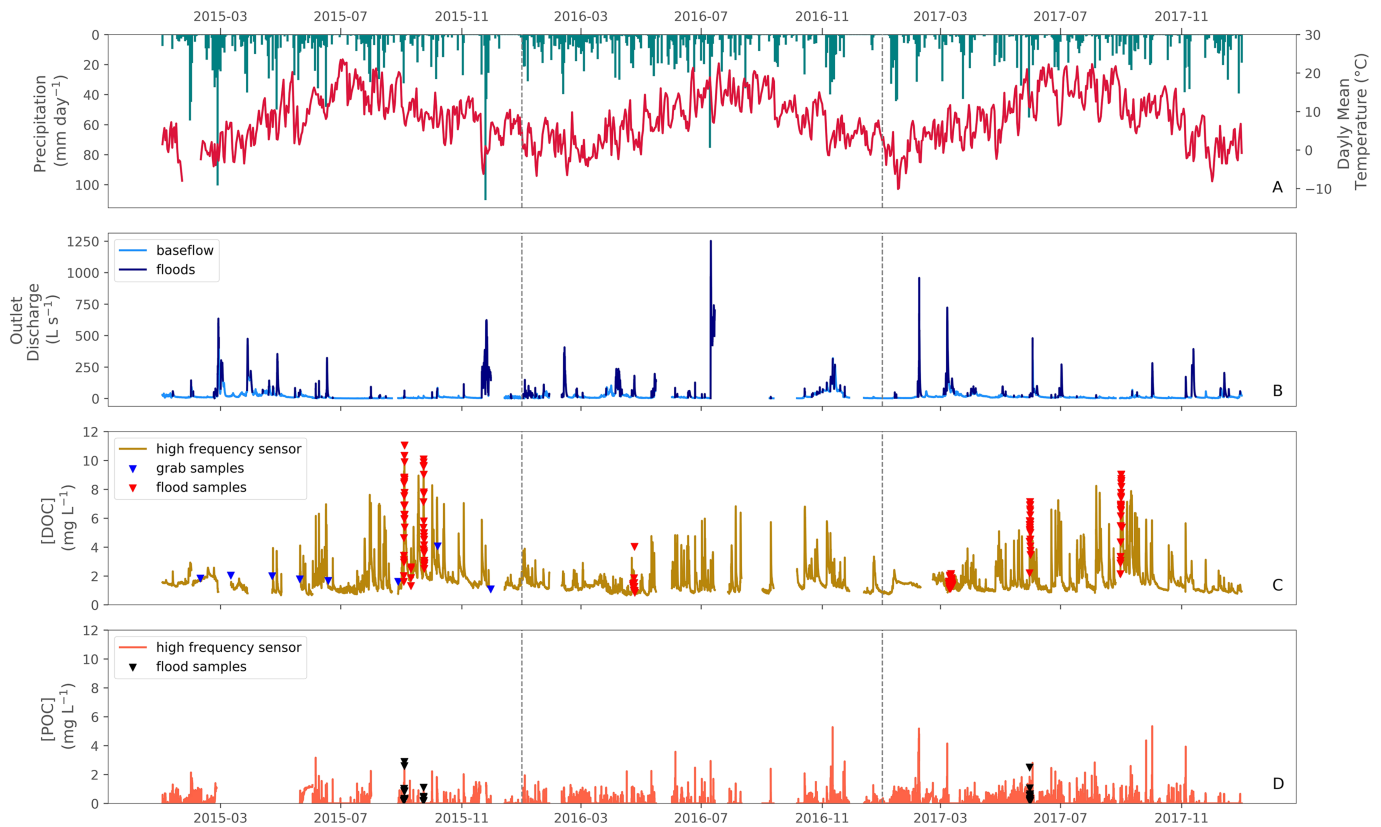
Figure 2. Precipitation and air temperature (a), discharge (b), high-frequency DOC concentration (c), and high-frequency POC concentration (d) time series observed at the outlet of the Bernadouze peatland over 3 years (1 January 2015 to 31 December 2017). The vertical grey lines represent a change of year. The dark blue periods on the discharge signal represent floods. Blue and red triangles in timeline (c) refer to DOC concentration measured in grab water samples and automated flood samples respectively. Black triangles in timeline (d) refer to POC concentration measured in automated flood samples.
