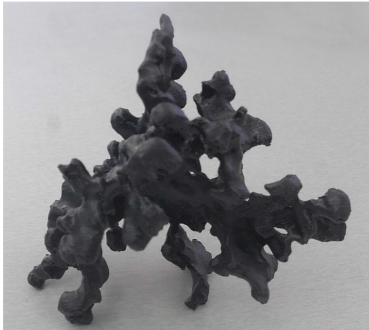
Figure 7 – Photograph of a 3D printing of graphite in a compacted graphite eutectic cell. The model was built from a tomographic study [10].
