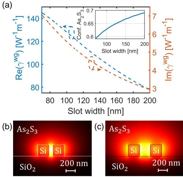
**Fig. 2.** (a) Simulated modal real (left axis) and imaginary (right axis) effective waveguide nonlinear susceptibility of hybrid  $As_2S_3$ -Silicon waveguides as a function of slot width. Inset: modal confinement factor in  $As_2S_3$ . TE-polarized modal profile for 70 nm (b) and 200 nm (c) slot widths.
