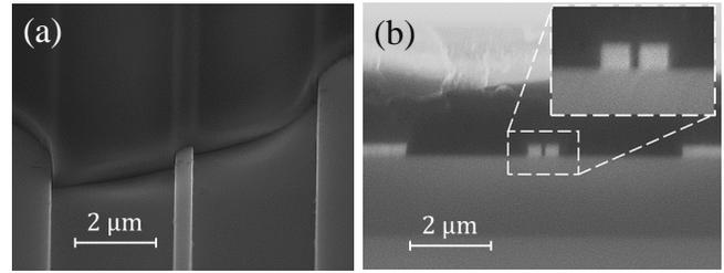
**Fig. 1.** Hybrid  $As_2S_3$ -on-Silicon waveguide platform. (a) SEM image of a Si strip waveguide covered with annealed  $As_2S_3$  glass. (b) SEM image of hybrid slot waveguide with 70 nm slot width and 220 nm  $\times$  220 nm Si rails, showing complete filling of the slot by  $As_2S_3$  after thermal treatment.
