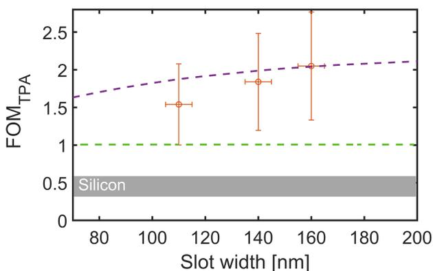
**Fig. 4.** Simulated TPA figure of merit ( $FOM_{TPA}$ ) as a function of the slot width (dashed purple line). Experimentally measured values for three different slot widths are also displayed. The olive-colored dashed horizontal line marks the threshold value of  $FOM_{TPA} = 1$ , and the gray bar corresponds to the typical  $FOM_{TPA}$  range in silicon waveguides.
