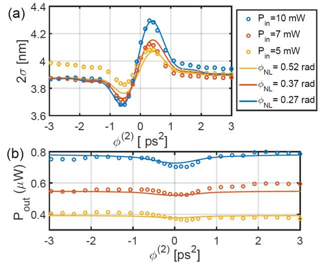
**Fig. 3.** D-Scan characterization of the waveguide with slot size 160 nm and propagation length of 0.85 mm. Measured (open circles) and simulated (solid line) spectral root mean squared linewidth ( $2\sigma$ ) (a) and output power (b) as a function of the second order dispersion  $\phi^{(2)}$  for three different average input powers.
