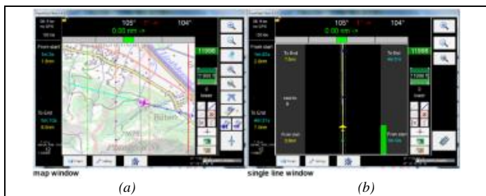
Fig. 9. Operator (a) and Pilot (b) real time trajectory display
