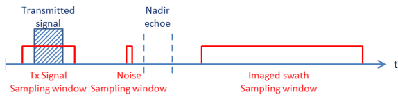
Fig. 3. Multi-sampling window principle
