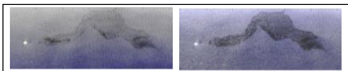
Fig. 12. L (left) and X (right) Band full polarization SAR image of non-hydrocarbon pollutants
