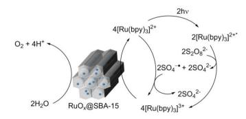
**Figure 4.** RuO<sub>2</sub>@SBA-15 system designed for OER photocatalysis in the presence of  $[Ru(bpy)_3]^{2+}$  as PS and persulfate as SEA reported by Ren and co-workers. Adapted from ref. [61].
