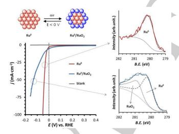
**Figure 7.** Polarization curves in a 1 M  $H_2SO_4$  solution at 10 mV·s<sup>-1</sup> and XPS data of metallic PP-Ru NPs and their Ru(0)/RuO<sub>2</sub> surface-passivated counterpart formed upon air exposure. Adapted from ref. [74].
