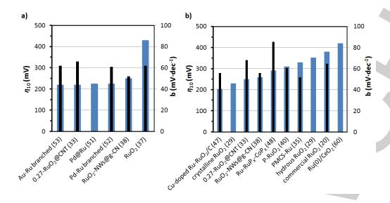
Figure 2. η10 (blue) and Tafel slope b (black) for the most relevant OER electrocatalysts in (a) acidic and (b) alkaline aqueous solution.
