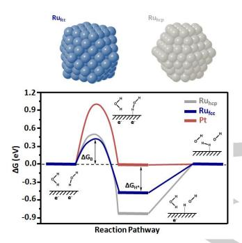
**Figure 9.** Top: Representation of the anomalous fcc-Ru phase (left) and the habitual hcp-Ru phase (right). Bottom: Gibbs free energy diagram of HER on Ru<sub>fcc</sub> (blue), Ru<sub>hcp</sub> (grey) and Pt (red) surfaces as reported by Qiao *et al.* [88].  $\Delta G_{H^*}$  corresponds to H adsorption free energy and  $\Delta G_B$  corresponds to water dissociation free energy barrier. Adapted from ref. [88].
