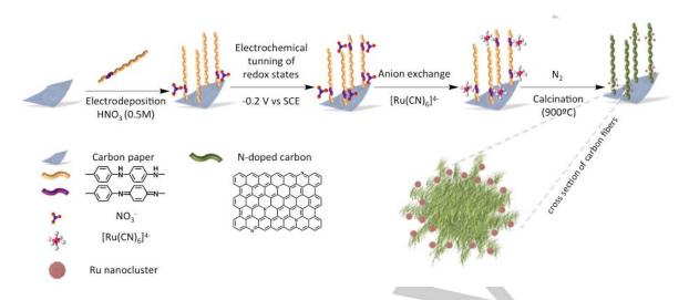
Figure 8. Schematic representation of the synthesis of the hierarchically-ordered N-doped carbon electrode containing 1.6 nm hcp-Ru nanoclusters (Ru@NC) reported by Yamauchi et al.[82] Color code: reduced polyaniline fibers, yellow; oxidised polyaniline fibers, violet.
