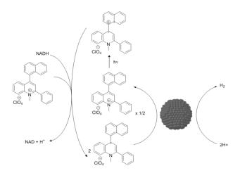
**Scheme 1.** Schematic representation of the electron transfer processes involved in photocatalytic hydrogen evolution promoted by Ru NPs in the presence of the QuPh<sup>+</sup>-NA organic donor-acceptor photoabsorber described by Fukuzumi et al. Adapted from ref. [112].
