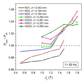
Fig. 1. Ratio of the Epstein to the effective ("true") power loss figure  $P_{\text{Epst}}/P_{\text{eff}}$  at 50 Hz measured in different types of non-oriented and grain-oriented steel sheets.  $P_{\text{eff}}(J_p)$  is obtained by precise local measurement of magnetic field strength and flux density.
