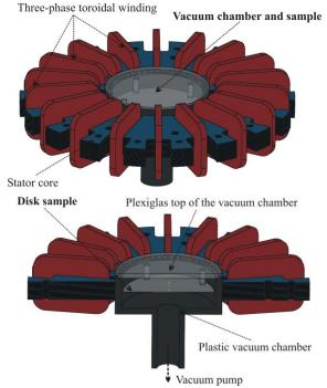
Fig. 15. Front and cross-sectional views of the high-flux density magnetizer. It holds the vacuum chamber employed for emulating quasi-adiabatic conditions during the measurement of the magnetic power loss with the thermometric method.
