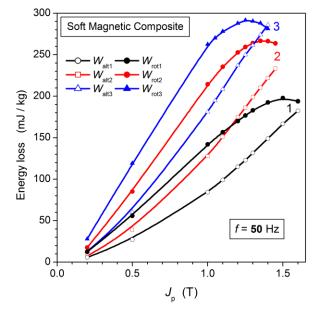
Fig. 20. Alternating  $W_{alt}$  and rotational  $W_{rot}$  energy loss measured at 50 Hz in three different types of Fe-based Soft Magnetic Composites. They are subjected to different preparation treatments, leading to different mass densities  $\delta$ . They attain the values:  $\delta_1 = 7450 \text{ kg/m}^3$ ,  $\delta_2 = 7260 \text{ kg/m}^3$ ,  $\delta_3 = 7110 \text{ kg/m}^3$ .
