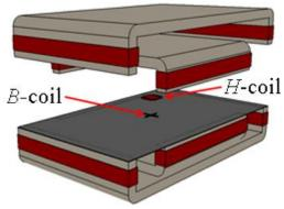
Fig. 8. Example of Vertical Rotational Single Sheet Tester [54].
