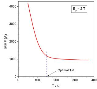
Fig. 16. Magnetomotive force per slot required to reach  $B_p = 2$  T at the center of the 0.20 mm thick disk sample as a function of the ratio T/d between axial height of the magnetizer and sample thickness.
