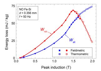
Fig. 21. Alternating  $W_{alt}$  and rotational  $W_{rot}$  energy losses in NO Fe-Si sheets measured at 50 Hz up to peak flux density  $B_p = 2.0$  T ( $J_p = 1.95$  T).
