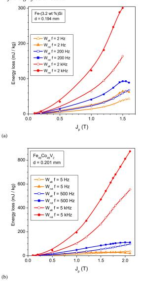
Fig. 18. Alternating  $W_{alt}$  and rotational  $W_{rot}$  energy losses measured with the use of the high-frequency RSST magnetizer in Fe-Si (a) and Fe-Co (b) non-oriented steels sheets up to the kHz range.
