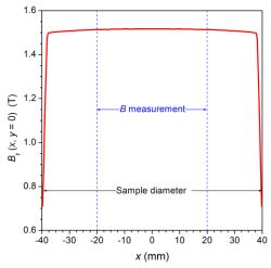
Fig. 13. Behavior of the magnetic flux density  $B_y(x, y = 0)$  across the 80 mm *x*-diameter of the non-oriented Fe-Si disk sample calculated for alternating magnetic field strength directed along the *y*-diameter. The *B*-measuring region is restricted to the -20 mm  $\le x \le 20$  mm region. The relative difference between  $B_y(0,0)$  and  $B_y(\pm 20 \text{ mm},0)$  is equal to 0.2%.
