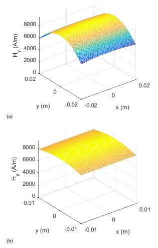
Fig. 14: Condition  $B_x=0$ ,  $B_y=1.5$  T, as in Fig. 12. a) Magnetic field strength homogeneity  $H_y(x,y)$  calculated by FEM analysis on the sample
