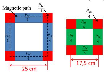
Fig. 3. Two Epstein frames with different limb lengths have been employed to determine the effective magnetic path length  $l_{\text{eff}}(J_p)$ . Its derivation relies on the assumption that the power loss in the corner regions is independent of the frame size [29][30].
