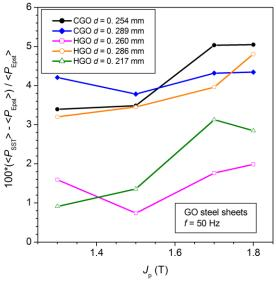
Fig. 5. The loss figure measured with the SST method  $P_{SST}$  (IEC60404-3) in CGO and HGO alloys is higher (~1 % - ~5 %) than the same quantity ( $P_{Epsl}$ ) measured using the Epstein frame (IEC60404-2) (adapted from [8], where the symbol <.> means the mean result between the different laboratories of the international comparison).
