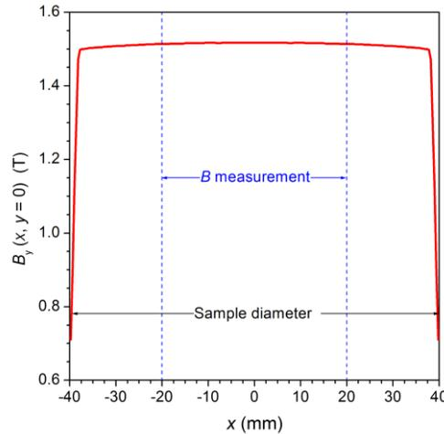
Fig. 13. Behavior of the magnetic flux density  $B_y(x, y = 0)$  across the 80 mm  $x$ -diameter of the non-oriented Fe-Si disk sample calculated for alternating magnetic field strength directed along the  $y$ -diameter. The  $B$ -measuring region is restricted to the  $-20 \text{ mm} \leq x \leq 20 \text{ mm}$  region. The relative difference between  $B_y(0,0)$  and  $B_y(\pm 20 \text{ mm}, 0)$  is equal to 0.2%.
