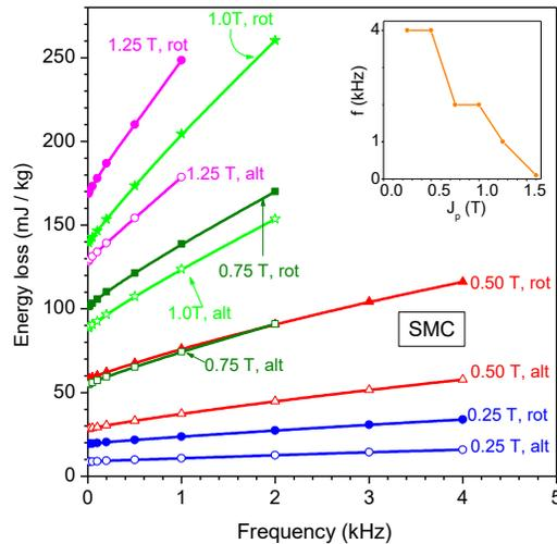
Fig. 19. Broadband energy loss under alternating and circular magnetic polarization measured with the high-frequency RSST in a Soft Magnetic Composite. The curve shown in the inset roughly delimits the accessible  $(f, J_p)$  measuring domain.
