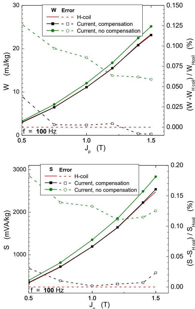
Fig. 7. Energy loss  $W$  and apparent power  $S$  are measured in GO steel sheets using the newly developed permeameter with and without compensation and with the  $H$ -coil method. The measurements are made at 100 Hz as a function of the peak polarization  $J_p$ . Compensation leads to drastic reduction of the discrepancies existing between the results obtained with the uncompensated permeameter and the  $H$ -coil method.
