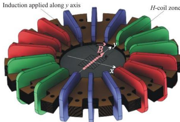
Fig. 12. An axis system  $x$ - $y$  is defined on the sample surface. The three-phase currents are set in such a way that an alternating flux density of peak value  $B_p = 1.5 \text{ T}$  is established along the  $y$  axis. The shadowed 20 mm square region centered on the sample surface is the  $H$ -coil zone.
