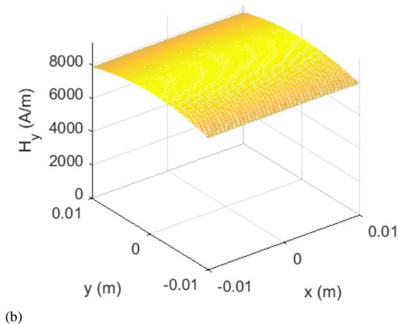
Fig. 14: Condition  $B_x=0, B_y=1.5$  T, as in Fig. 12. a) Magnetic field strength homogeneity  $H_y(x,y)$  calculated by FEM analysis on the sample
