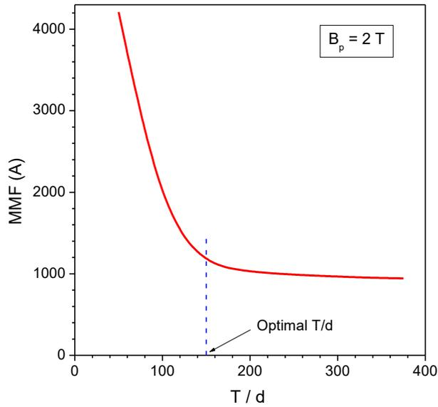
Fig. 16. Magnetomotive force per slot required to reach  $B_p = 2$  T at the center of the 0.20 mm thick disk sample as a function of the ratio  $T/d$  between axial height of the magnetizer and sample thickness.
