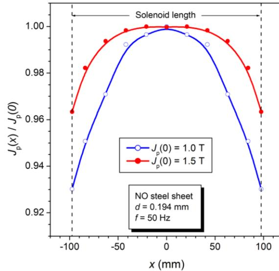
Fig. 4. Reduced value  $J_p(x) / J_p(0)$  of the peak polarization in NO Fe-Si strip samples across the limb length  $l_0 = 195$  mm (the length covered by the windings, with center at  $x = 0$ ) of a standard Epstein frame.  $J_p(x)$  is measured by means of a localized pickup coil, collinear with a narrow  $H$ -coil, allowing for simultaneous measurement of  $P_{\text{Epst}}$  and the local power loss  $P_{\text{eff}}(x)$  [10].
