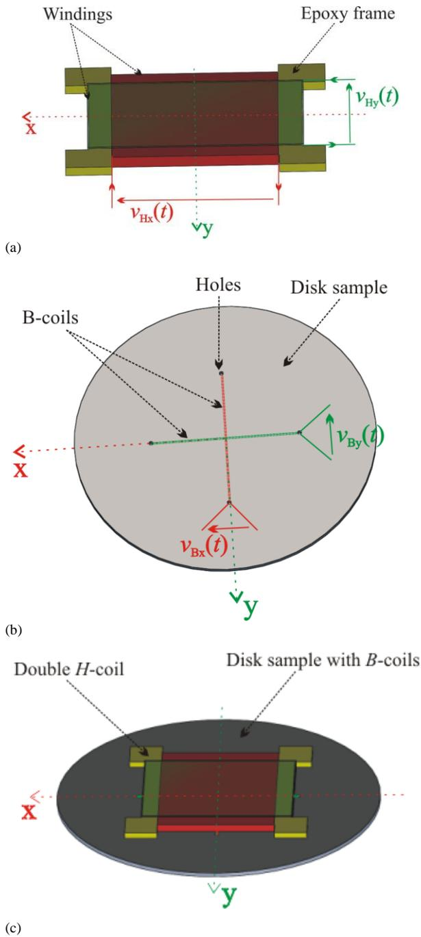
Fig. 9. Arrangement of  $H$ - and  $B$ - windings for the 2D characterization of magnetic sheets. a) Crossed  $H$ -coils for the measurement of  $(dH_x/dt, dH_y/dt)$ ; b) Crossed  $B$ -windings, made of few turns threaded through small holes, providing  $(dB_x/dt, dB_z/dt)$ ; c) Final arrangement of the  $H$ - and  $B$ - coils for the fieldmetric measurement of 2D hysteresis loops and losses.
