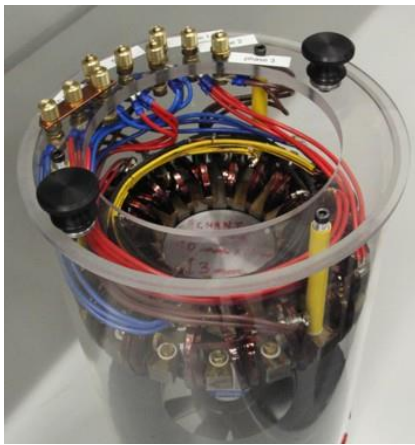
Fig. 11. Three phase magnetizer designed for 2D magnetic measurements up to the kHz range. a) Schematic view and 3D FEM model. b) Assembled setup with test sample (adapted from [89]).
