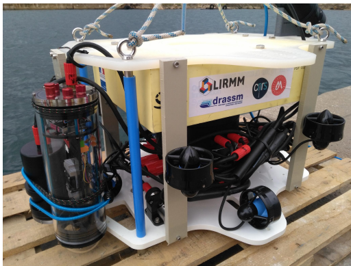
Figure 3. The Remotely Operated Vehicle Dumbo and the acquisition system A, used to record the harbor sequences.
