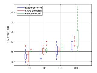
Figure 2: Effects of the earmuff, assessed by the three different methods as the difference between the masked thresholds with and without HPD.
