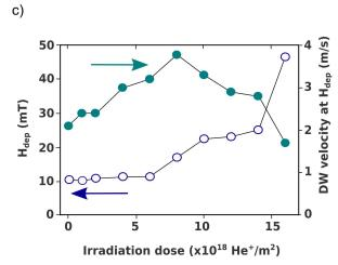
FIG. 1: (a) Sketch depicting the perpendicularly magnetised CoFeB stack and the effect of  $\mathrm{He}^+$  irradiation at the interfaces. (b) Anisotropy field  $H_k$  as a function of the irradiation dose. (c) Depinning field  $H_{dep}$  (blue circles, left axis) and its corresponding DW velocity  $v(H_{dep})$  (cyan circles, right axis) as a function of irradiation dose.
