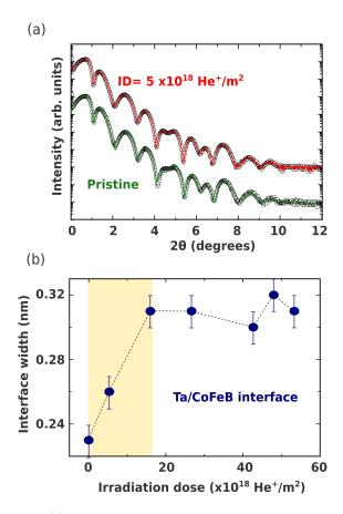
FIG. 3: (a) X-ray reflectivity profiles for a pristine and an irradiated films at ID=  $5\times 10^{18}~{\rm He^+/m^2}$ , the corresponding model is plotted as solid lines. (b) Width of the Ta/CoFeB interface as a function of the irradiation dose.
