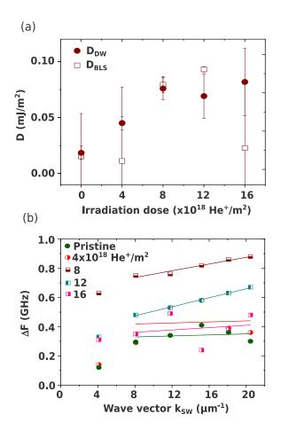
FIG. 5: (a) DMI constant D as a function of the irradiation dose obtained by DW motion measurements and BLS. (b)  $\Delta F$  as a function of the wave vector for pristine and irradiated films with ID= 2, 4, 8, 12 and 16x  $10^{18} \text{He}^+/\text{m}^2$ . Solid lines linear fits of the high  $k_{sw}$  regime from which the  $D_{BLS}$  values presented in (a) were extracted.
