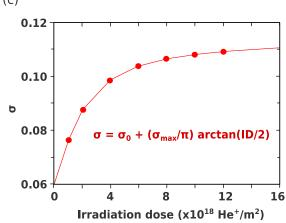
FIG. 6: Micromagnetic simulations considering the irradiation induced changes in the intrinsic parameters with (a) a constant disorder and (b) an ID dependent disorder. The simulated disorder variation with ID is plotted in (c).
