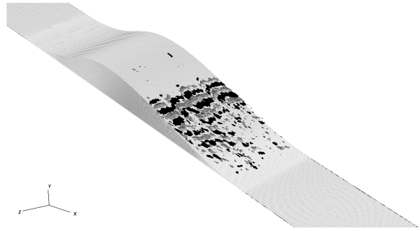
Figure 15: The DMD mode for St = 2 computed from the flow around the bump, illustrated using two opposite contours of the perpendicular velocity component \mathbf{u}_\perp .
