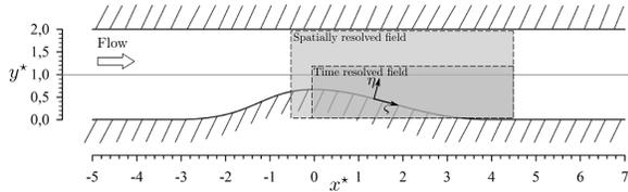
Figure 2: Test section containing the two-dimensional bump geometry and the PIV fields of interest. The symbol  $*$  denotes the half height normalization.  $\eta$  represents the direction of the local outward normal of the surface and  $\zeta$  the tangential direction.
