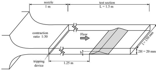
Figure 1: 3D view of the channel setup.
