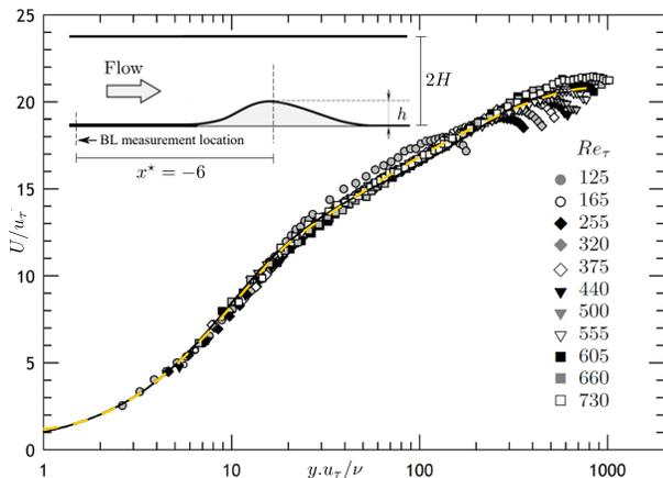
Figure 3: Profiles of the streamwise velocity against the wall-normal coordinate for various Reynolds-numbers. Dashed line represents DNS results of [26] at  $Re_\tau = 617$
