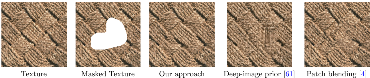
Fig. 17: Textural inpainting comparison. In this example we compare our approach with Deep image prior [61] (which optimizes a deep neural network with skipping connection to generate the masked image using Mean Square Error criterion) and with [4], where patches from the uncovered part of the image are used to fill in the masked domain and blended to avoid blocking artifacts. Notice that the available textural content is better represented with our approach since it is inherently designed to respect the patch distribution.
