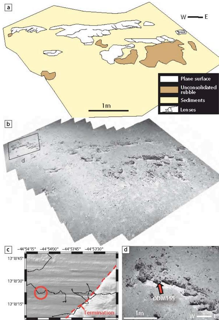
**Figure S5:** (a) Geological interpretation of (b) videomosaic ROV high-resolution video survey of outcrop #6 (see location in **Figure 1b**). (c) Shaded relief microbathymetry of outcrop #2. The outcrop location is indicated with a red circle, the corrugated surface termination is shown with a dotted red line, and the ROV paths with white lines. (d) Close up on the location of ODM155 (red arrow).
