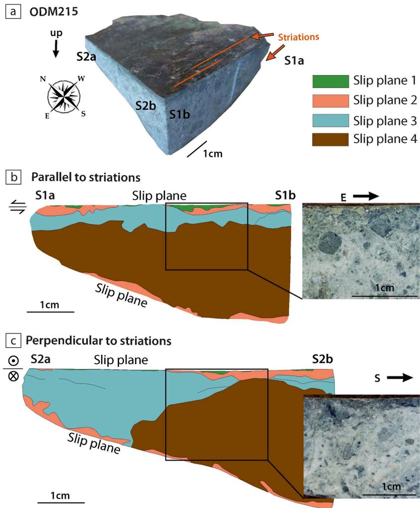
**Figure S9:** (a) Location of the two sections of the oriented ODM215 fault rock: one parallel (b) and the other perpendicular (c) to striation direction. (b-c) Interpretation of cut surfaces whose structures are shown in the insets. Different slip zones are distinguished by their color and differences in clast content and size. Internal structures are indicated by black lines.
