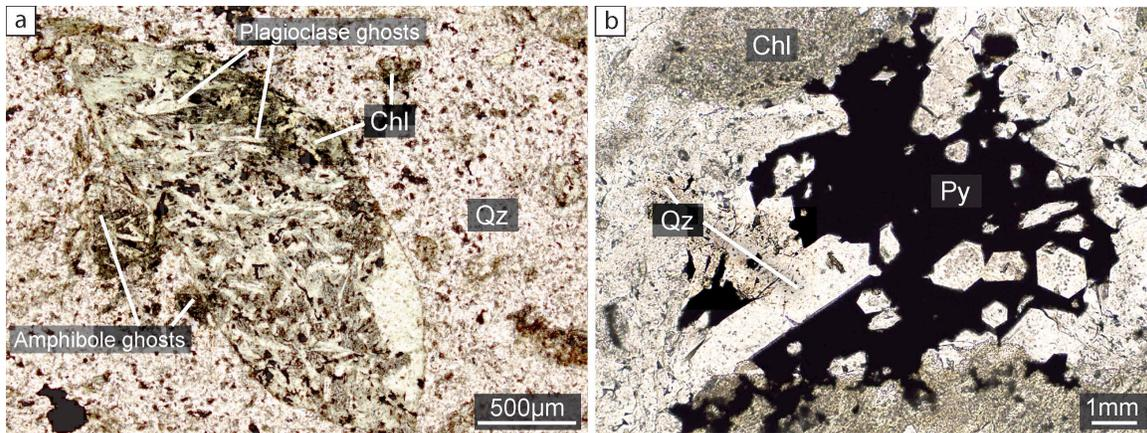
**Figure S7:** Microphotographs of highly silicified sample ODM218 under parallel nicols of: (a) a chloritized clast where ghosts of primary minerals can be recognized by their texture and similarity with clasts from moderately silicified samples (**Figure 7a**); (b) Intergrowth of pyrite and quartz.
