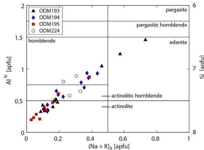
**Figure 7.** Composition of amphibole for four moderately silicified mafic samples containing rare chlorite in the matrix and clasts (ODM193, ODM194, and ODM224), and chlorite commonly found in both matrix and clasts (ODM195). The increase in chlorite contents is associated with a general shift toward amphibole compositions from hornblende to actinolite, corresponding to decreasing temperatures.
