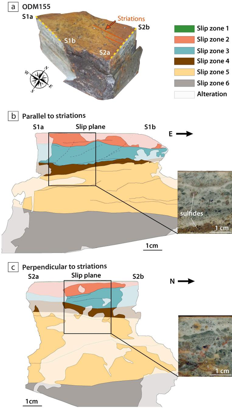
**Figure S8:** (a) Location of the two sections of the oriented ODM155 fault rock: one parallel (b) and the other perpendicular (c) to striation direction. (b-c) Interpretation of cut surfaces whose structures are shown in the insets. Different slip zones are distinguished by their color and clast content. Internal structures are indicated by black lines, and alteration zones and halo by the whiter zones, primarily along the borders of the sample.
