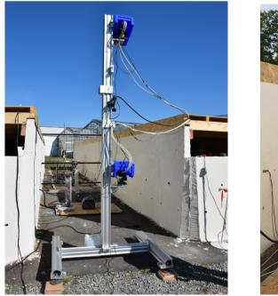
(a) Stereo-PIV setup arrangement
